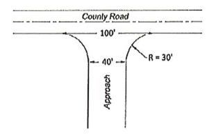
3. If a property is higher or lower than the adjacent public roadway, the approach coming onto the roadway shall not have more than a three percent (3%) grade connecting it to the roadway for a distance of not less than thirty feet (30'), and the approach leading to the roadway must allow the vehicle to stop on the thirty-foot (30') approach at the three percent (3%) grade.
